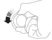
Unscrew the bulb cover by turning counter clockwise. It may be very stiff.
